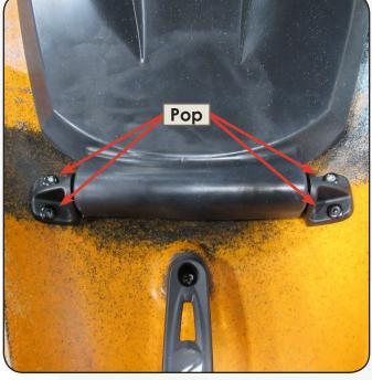
5. Insert the Cherry Rivets(B) into each hole and while pressing down on each Hatch Hinge, pop the rivets with your Rivet Gun.
